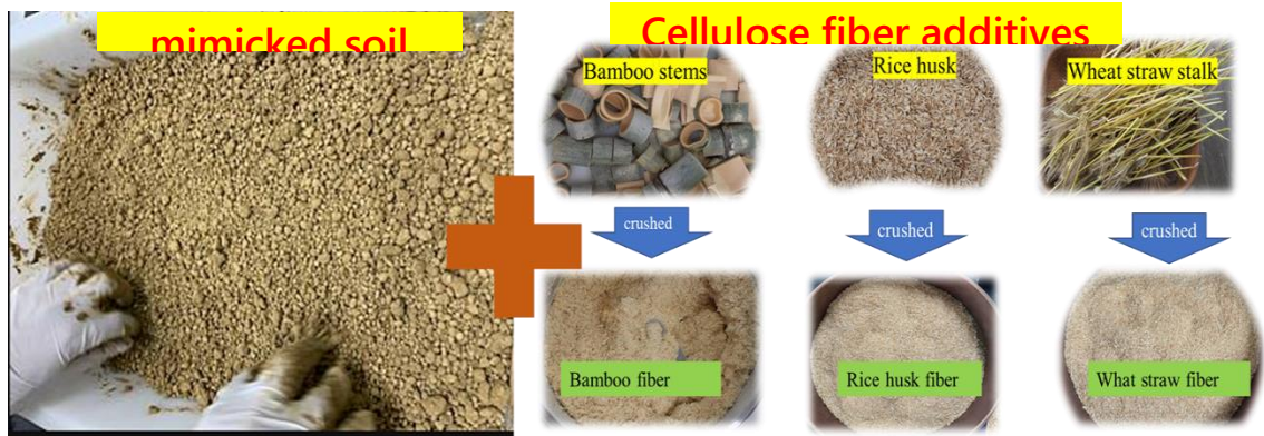
Figure 2: Stabilization process of the pseudo-expansive soil with cellulose-based fibers
